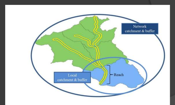
Figure 2. Stream reaches and local and network catchments and buffers (modified from Wang et al. 2011).
